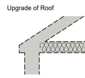
Existing roof structure to be exposed by contractor. All existing insulation to be removed and replaced with min 400mm mineral wool.
